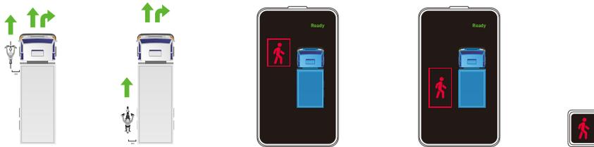
⑤ Speed at  $0 < \text{speed} \leq 30 \text{ km/h}$ , when VRU are detected by the left AI camera, the distance is within 1m, At this time, when the left turn signal is turned on or the steering wheel is turned, the display shows a red icon, the left A-pillar LED gives a red flashes, and the display emits an audible warning.
